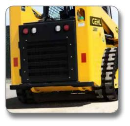
COUNTERWEIGHT/BUMPER Gain extra tipping capacity while offering increased rear protection. Increases rated operating capacity by 100 lbs. (46 kg) and adds 1.5" (38 mm) to overall length.
