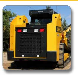
COUNTERWEIGHT/BUMPER Gain extra tipping capacity while offering increased rear protection.
